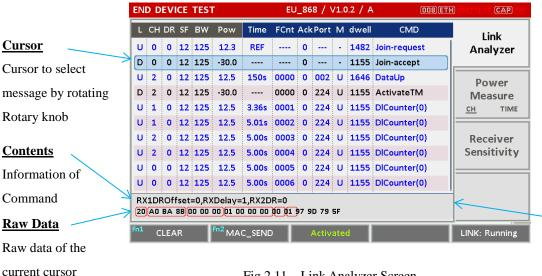
Fig 2.11 Link Analyzer Screen
