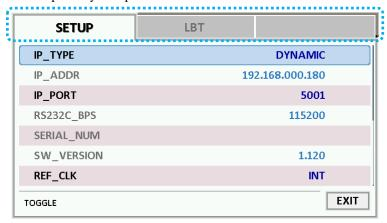
Fig 2.10 System Configuration Screen
