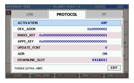
Fig 3.25 Parameters for ABP (LoRaWAN V1.0)
