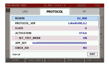
Fig 2.5 Parameter Configuration Screen
