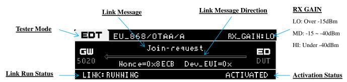
Fig A.4 RWC5020M Screen in running state
