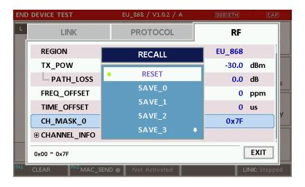
Fig 2.21 Screen of Parameter Configuration RECALL
