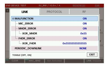
Fig 3.31 Malfunction configuration parameters
