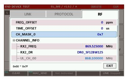
Fig 3.7 Channel Information in RF Parameters
