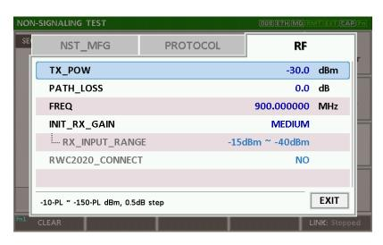
Fig 3.44 RF Parameters for MFG Test
