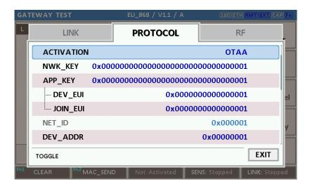
Fig 3.22 Parameters for OTAA (LoRaWAN V1.1)
