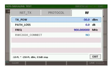
Fig 3.32 RF Parameters for Signal Generator
